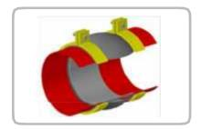
Convoluted fabric expansion joints are attached directly onto the outside of the duct using clamping bands normally used for:
